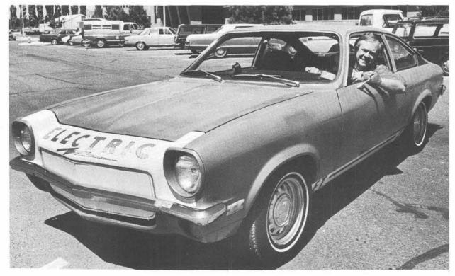
DICK BASSETT (2354) occasionally drives his home-built electric Vega to work (when he can talk his wife out of it). It's a high performance (60 mph with quick acceleration) vehicle with limited range (35 miles on a charge) and costs between 134 and 3 cents per mile, depending on fuel adjustments and electric rates.
